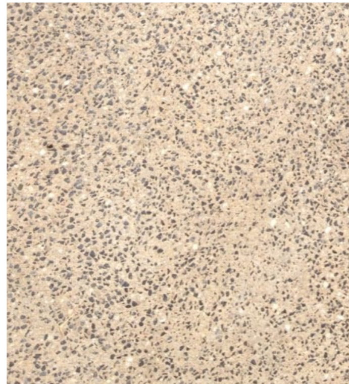
Exposed aggregate concrete paving Exposed aggregate mix : 50% bluestone; 50% 10mm Mount View quarries white pebble. Concrete available from: Vickery Bros. Pty Ltd Contact: 03 5575 2777 Pebbles available from: Horsham Concrete Contact: 03 5381 0831
