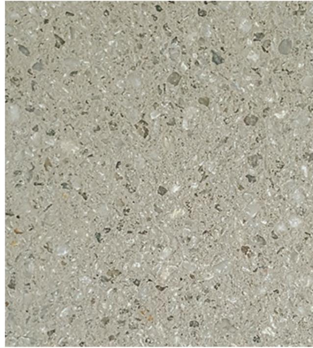
Feature pavement option - G2 Paver 'Hearth' by SVC or similar colour / texture lightly exposed aggregate concrete.
