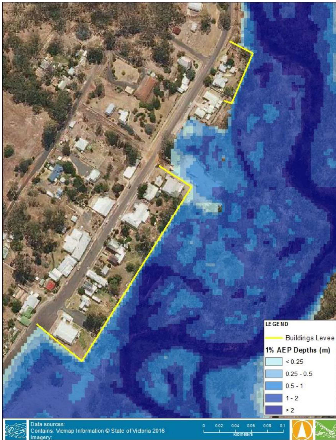
Figure 8-5 Buildings Levee Alignment and 1% AEP depths
