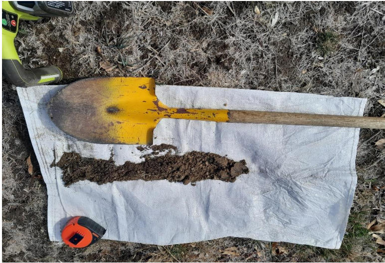
Soil Test: Horizon B 50-600mm Category 5 clay soil
