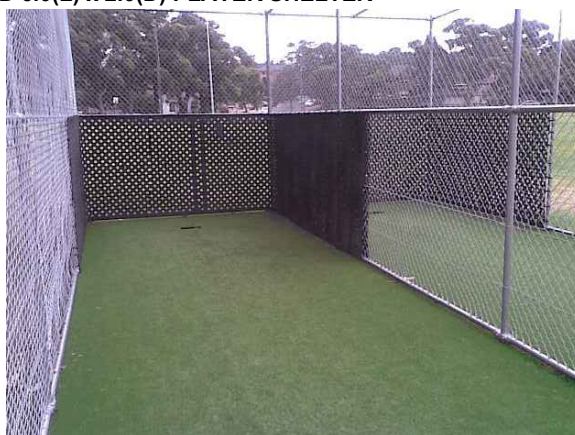
TYPICAL RUBBER BELTING - TO BE INSTALLED ALONG THE NORTH AND SOUTHERN SIDE OF FENCE - 61m
